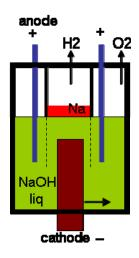
With Castner-Tiegel method, electrolysis is performed (0 to 20C) above the NaOH melting temperature (318C). Molten salt enables high ionic conduction.
