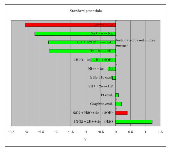
Standard potential for reduction (mainly from [2.1]). In red: main potentials for LiOH electrolysis, which difference is 3.44V. (For real activation potential, temperature should considered and potential for LiOH ionic separation should be added.)
