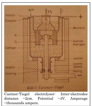
Metal sodium migrates to the top of the melt, and is separated from anode O2. Cathode is kept under sodium metal level to avoid short-circuits. Electrodes are separated by a dense iron net. Na is extracted from top, using a spoon with holes (continuous extraction through an hollow cathode is also possible). Production is continuous (continuous NaOH feeding). Away from electrodes, NaOH is kept unmelted, for sealing and thermal insulation.
